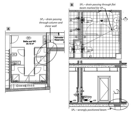
Figure 8: Examples of (A) SP<sub>2</sub> with hard clash, and (B) SP<sub>3</sub> and SP<sub>4</sub>.
