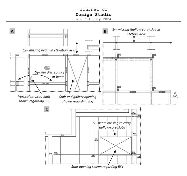
Figure 2: Examples of structural system design deficiencies.
