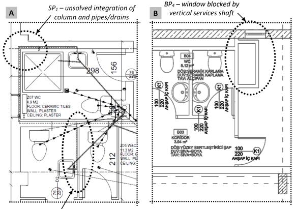
BP<sub>2</sub> – insufficient wall thickness to embed pipes/drains
